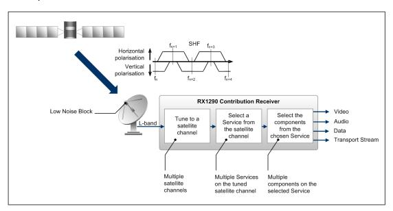
Figure 1.3 What the Satellite Receiver Does
